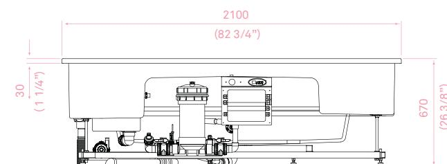
Tub with skimming lip, built with a special fiberglass / gelcoat anti-osmosis. Steel support frame resting on 8 adjustable feet. Water heating by heat-exchange system or electrical heating system.
