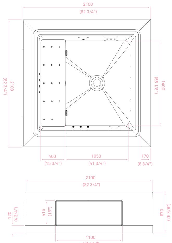
Tub with skimming lip, built with a special fiberglass/gelcoat anti–osmosis. Steel support frame resting on 8 adjustable feet. Aesthetic skirting with function of safety tank. Inox nozzles. Water heating heat-exchange system or electrical heating system.
