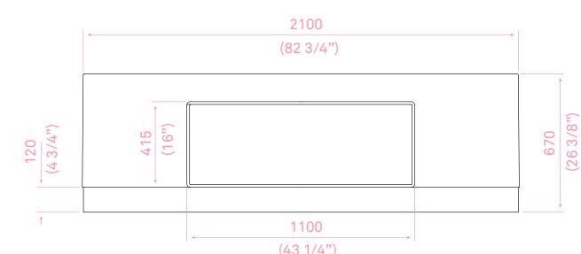
Tub with skimming lip, built with a special fiberglass/gelcoat anti-osmosis. Steel support frame resting on 8 adjustable feet. Aesthetic skirting with function of safety tank. Water heating by heat-exchange system or electrical heating system.
