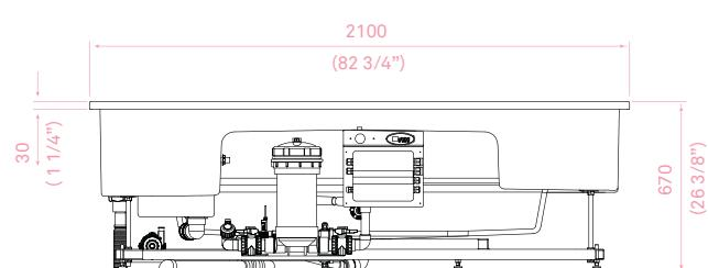
Tub with skimming lip, built in a special fiberglass/gelcoat anti–osmosis. Steel support frame resting on 8 adjustable feet. Inox nozzles. Water heating heat-exchange system or electrical heating system.
