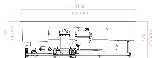
Tub with skimming lip, built with a special fiberglass/gelcoat anti-osmosis. Steel support frame resting on 8 adjustable feet. Inox nozzles. Water heating by heat-exchange system or electrical heating system.
